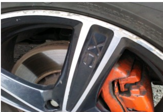
osf alloy corroded
