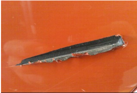
front bumper cracked
