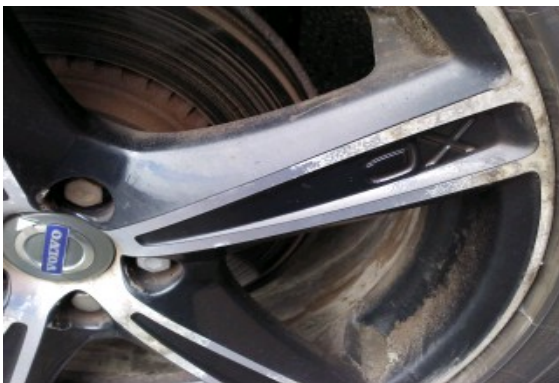
nsr alloy corroded
